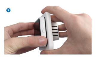
During removal or installation do not press the button on the side of the control panel. The power should be cut off from the thermostat prior to removal or installation of the control panel.
