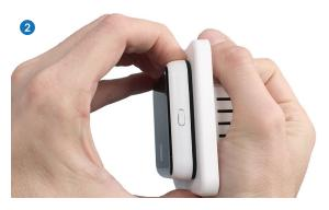
You can brace your thumb against the outter frame. However do not press down on the front of the panel or pry the sides of the panel as this may result in damaging the control panel or breaking the clips that hold it.
