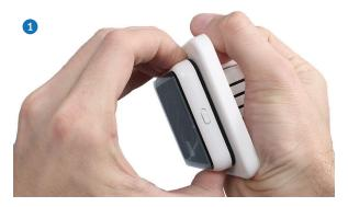
Grab hold of the control panel from the top and the bottom. Squeeze the the panel and pull it toward you. The Panel is held by a two stage clip for the bottom and the top. The first-time removal may be tougher and require a bit more force.
