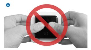
Under no circumstances, are you to press the centre of the control panel. This may cause permanent damage to the control panel.
