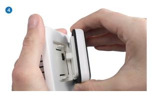
To re-install the control panel, align the connector with the outlet slot. The connector needs to be installed perfectly in line with the outlet. Do not use force when aligning the connector with the outlet.
